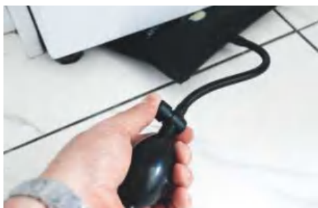
▲ The bulb is squeezed to inflate the bag as needed; even heavy weights are easily lifted
